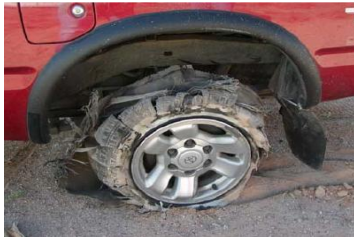
Figure 1: A failed pneumatic tyre
